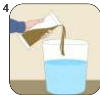
4 Mix the measured quantity of Cement Tonic-LW+ to the remaining gauging water in a bucket and stir thoroughly.
